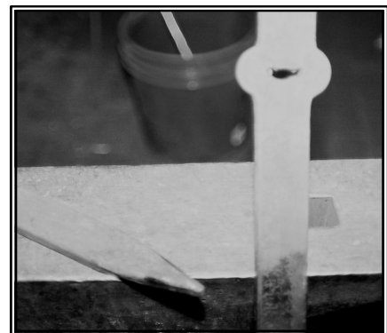
Figure 10 The Hole Parallel to the Bar Has Been Changed to an Opening Perpendicular to the Bar
