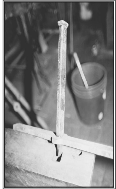
Figure 11 Drifting the Hole Perpendicular to the Bar
