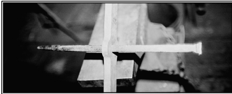
Figure 12 Hole Drifted to Full Dimensions
