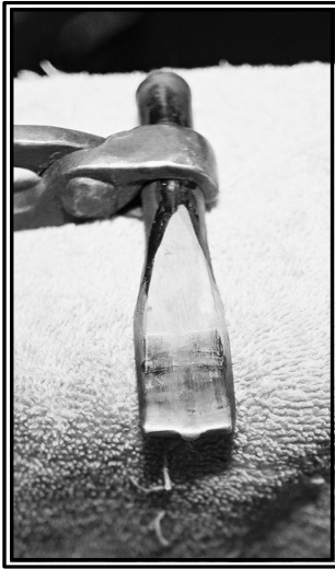
Figure 3 Slitting Chisel Note Center Point
