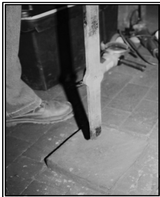
Fig 8 Upsetting Bar Using Floor Plate The Bar is Rotated 90° Between Strikes on Floor Plate to Maintain Even Upset
