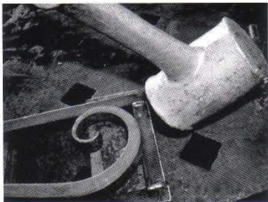
L: One method of shortening is to put the hot end in the box and hammer the cold end into position.
