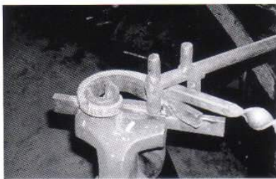
The tapered bar is wrapped around the tool, a bending fork is needed to keep from bending the bar at the twist..
