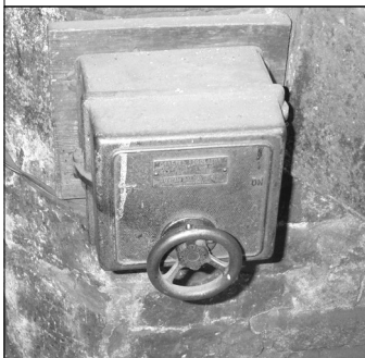
Forge blower speed is regulated by this antique rheostat.
