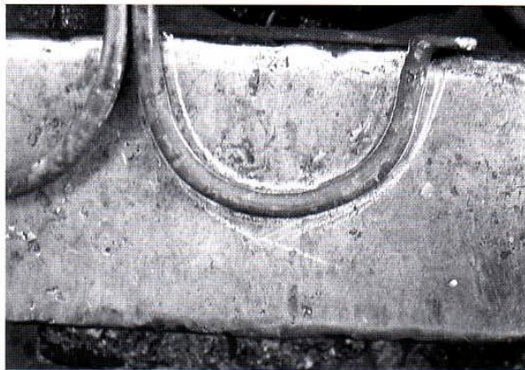
Matching the two curves with the aid of a soapstone.
