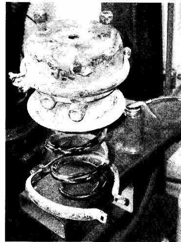
The parking brake chamber in the position when the retaining bolt was cut. The 15-lb. housing flew upward like a missile.
