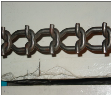
This chain was seen at the Soul'e Foundry in Meridian. The individual links separate to make the chain any length necessary.
