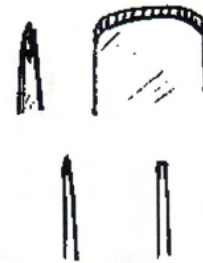
Enlarged view of liner chisel (top) and actual size of working end of liner (bottom).
