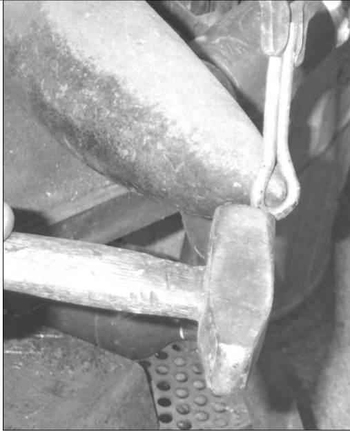
(1) Forming eye Starting with a piece of 1/4" rod about 12" long, form an eye resembling a big cotter pin. The inside diameter of the eye should be a smidgeon over 1/2" to allow both legs of another pin to pass through it.
